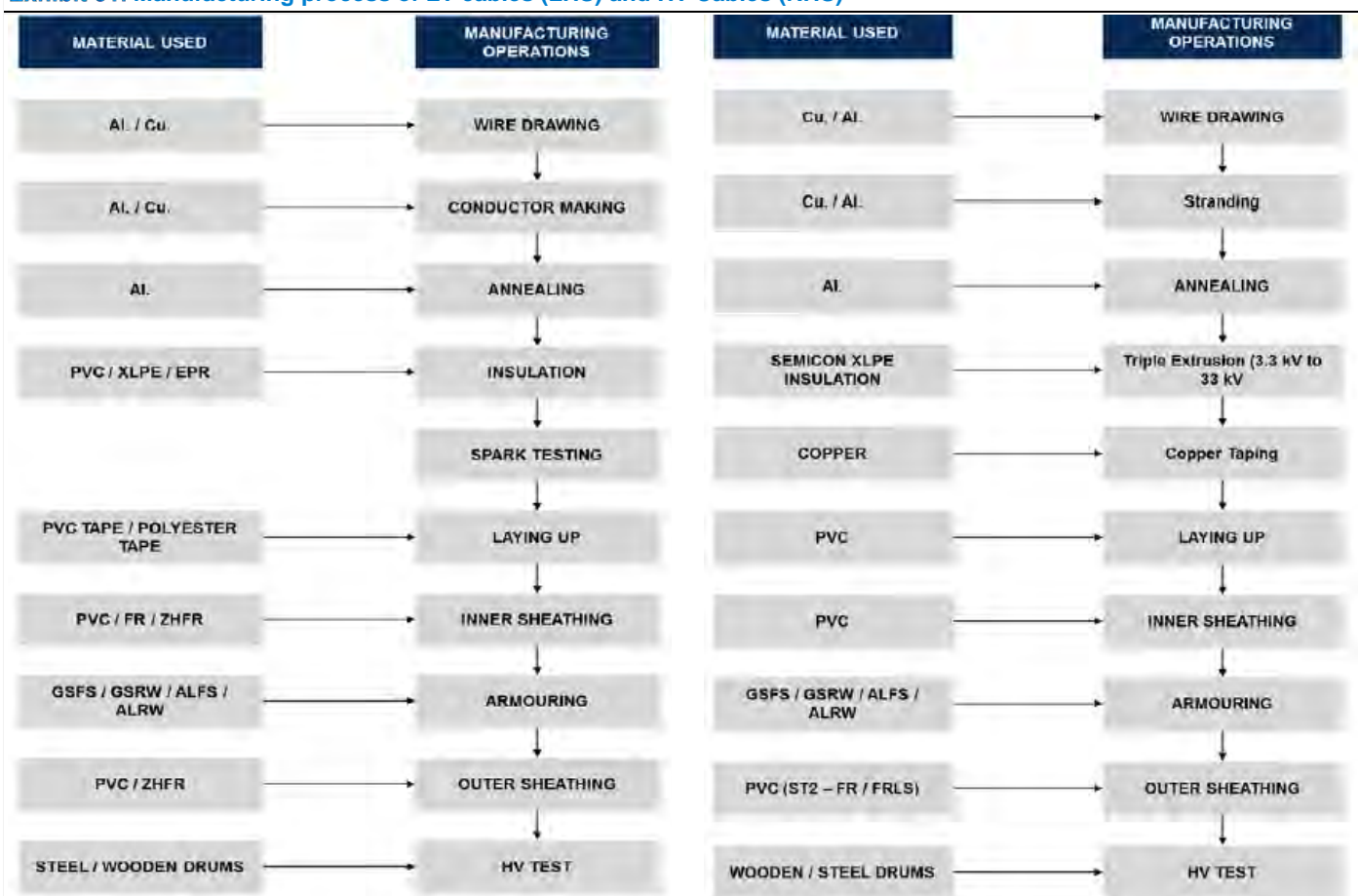
Exhibit 51: Manufacturing process of LT cables (LHS) and HT Cables (RHS)
