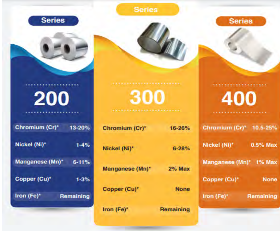
Exhibit 5: Composition of various types of stainless steel grades
