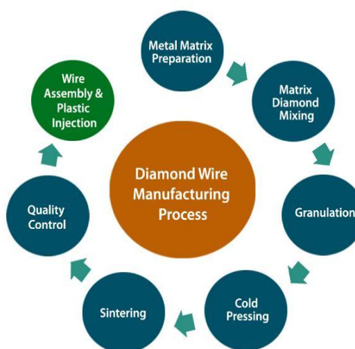
Exhibit 12: Process employed for manufacturing diamond wires
