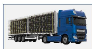
Type IV CNG Cylinder Cascades Lighter – Carries 220% More Gas
